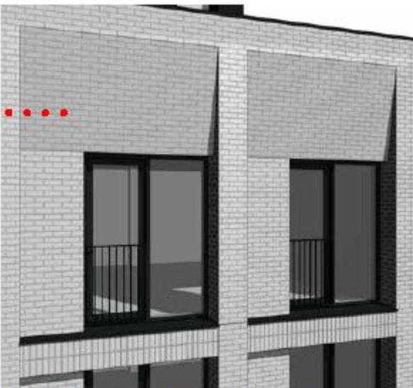
Brick soffit detail to Ellesmere Street Elevation
