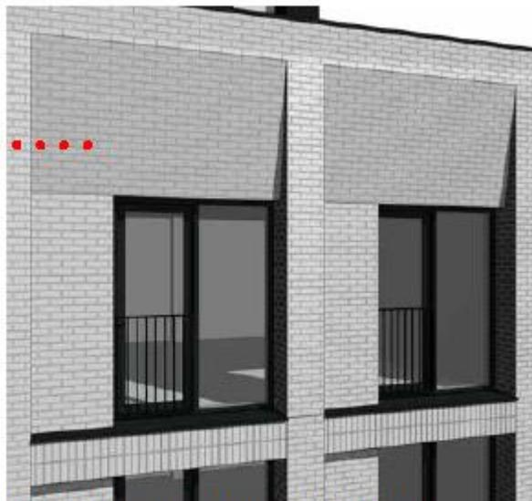
Brick soffit detail to Ellesmere Street Elevation
