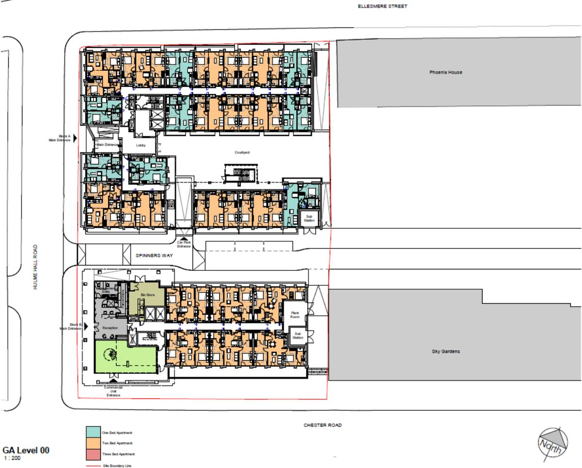
Vehicular access would be off Hulme Hall Road via Spinners Way, which would be part of a route created through the site. There would be an entrance ramp off Spinners Way to a basement under Block A which includes 27 parking spaces and a secure cycle store for 366 bikes. Three parking spaces would be provided on Spinners Way. Four of the basement spaces would be suitable for use by disabled people, equating to 13%. Two bin stores and plant would be in the basement.
