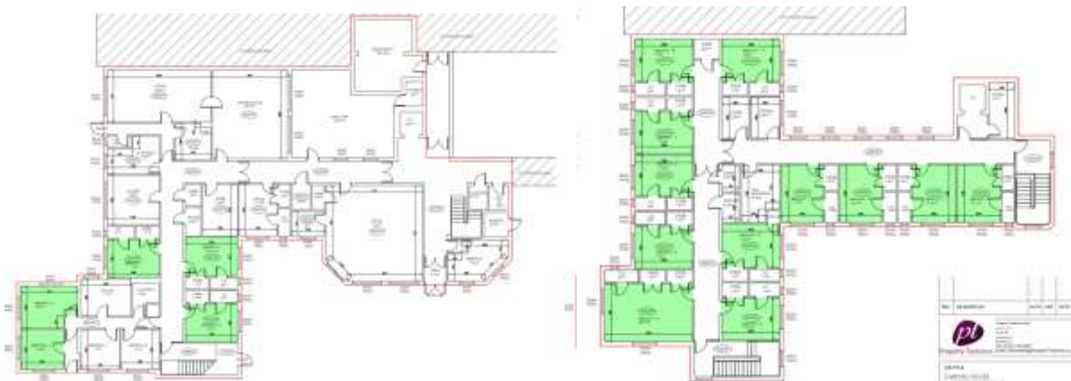
Proposed ground and first floor layout (Ancillary office to bedroom conversions are shown in green)
