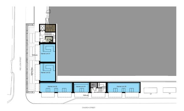
There would be a roof terrace with seating and tables for customers of the upper floor food units. The upper floor of unit 5 would be back-of-house or stock store. The final distribution and division of units would be determined with Manchester Markets. The units would be constructed from a mixture of pressed and flat sheet aluminium with set back coloured metal backed mesh shutters.
