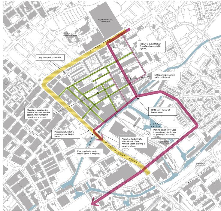
Figure 4.3: Plan showing critical section of GAS along which interventions are necessary
